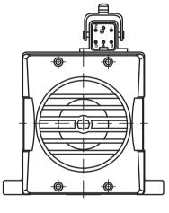
Special attention: thread locking adhesive shall be applied or the spring washer shall be added to prevent the looseness during the installation of the fastening screw!
