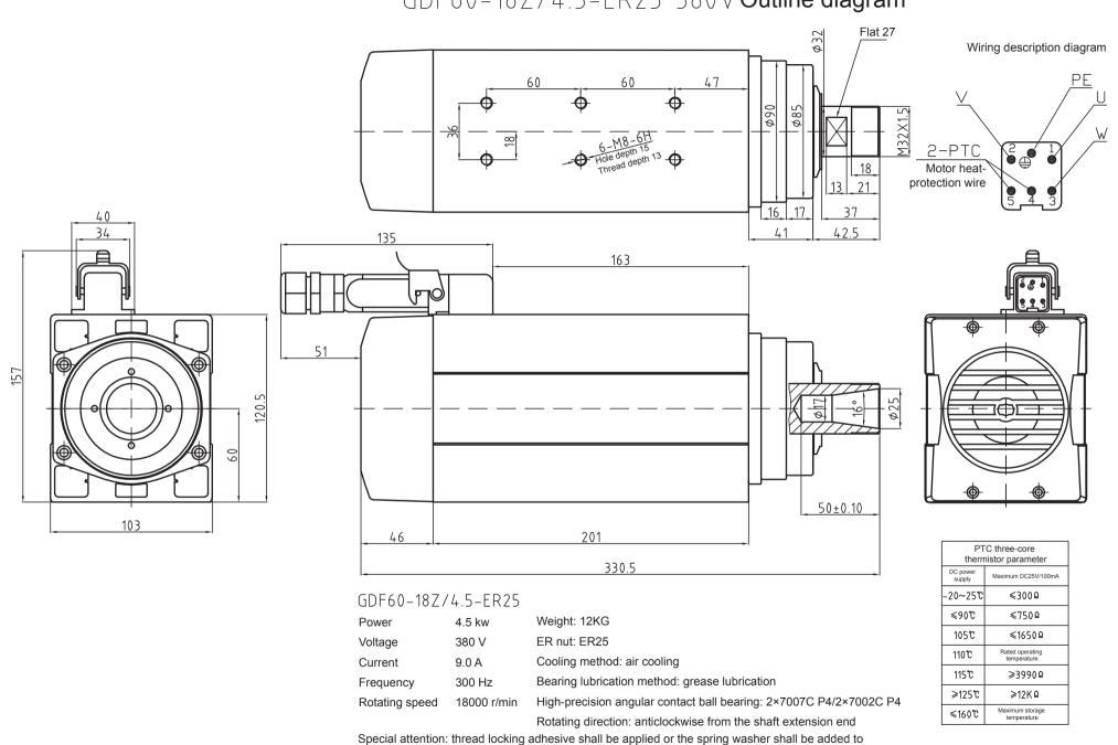
prevent the looseness during the installation of the fastening screw!
