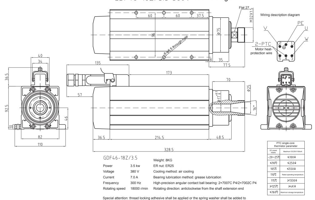
Special attention: thread locking adhesive shall be applied or the spring washer shall be added to prevent the looseness during the installation of the fastening screw!
