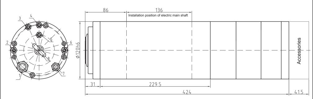
1: Power line Three-color lines connected with U, V and W phases/ yellow and green wires grounded Temperature control line 110°C thermistor two-phase connected with the temperature-control protector
