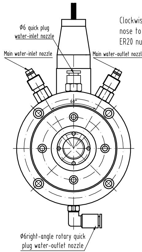
Clockwise rotation viewed from the spindle nose to the spindle at the rear end
